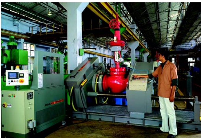
High Pressure Test Bench for testing valves upto 24" size
